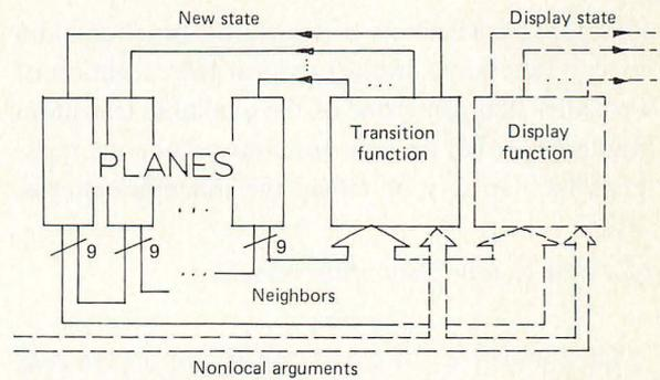
Fig. 1. CAM's basic computational loop (solid lines), with nonlocal arguments and display function (dashed lines).
