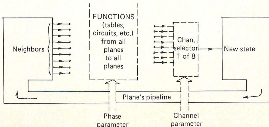
Fig. 2. CAM's pipeline (solid lines), with gap to be filled by the transition function. In the dashed portion, the channel selector connects the pipeline input to any one of 8 different sources, and the phase parameter can be used to modify the behavior of such sources. Any interactions between pipelines takes place in the "functions" box, where all of the random wiring is located.
