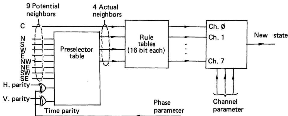
Fig. 3. Portion of CAM wired to run several rules based on the Margolus neighborhood. Neighbor “preselection” is done by a combination of hardware and table look-up, so as to permit use of smaller tables for the rules themselves. The phase bit determines whether a rule should execute forward or time-reversed.
